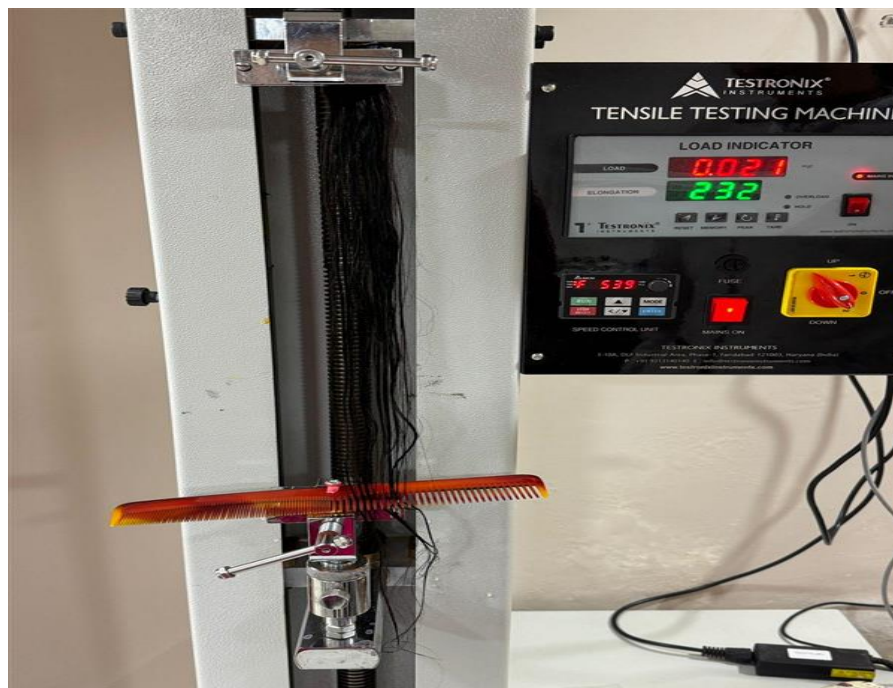
Figure 4: TESTRONIX Tensile Strength Tester Automatic Combing System
